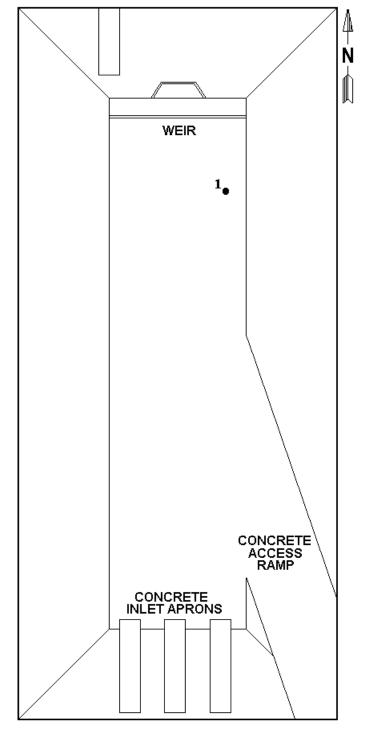
FIGURE 1. APPROXIMATE LOCATIONS OF LEAKS FOUND IN METAL CLEANING BASIN
